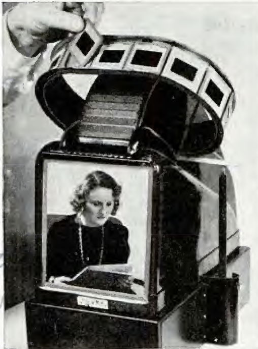
Rear view, left, shows viewing glass and the slide carrier. Right, projecting picture onto a screen
